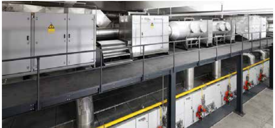
BRÜCKNER POWER-FRAME stenter with ECO-HEAT and ECO-AIR systems
